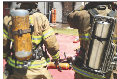
Firefighters testing liquid air pack vs. standard SCBA - Photo courtesy of CLSS
