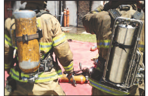
Firefighters testing liquid air pack vs. standard SCBA - Photo courtesy of CLSS
