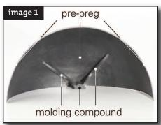
The combination of pre-preg and molding compound opens options for designing geometrically complex parts. The addition of ribs in the domed part produces a part with nonuniform deflection behavior (Image 1). A load placed directly on top of a rib produces less deflection than if the load is placed between the ribs (Image 2 and 3). While this behavior is expected, the degree by which it was manifest in this case demonstrates the significance of using geometry to alter the deflection of a part.
