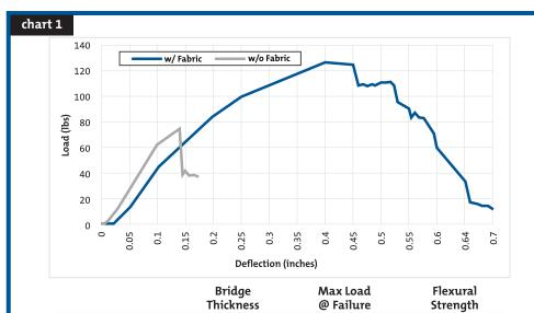
Note: The continuous fiber pre-preg did not break. The molding compound delaminated from the pre-preg.
