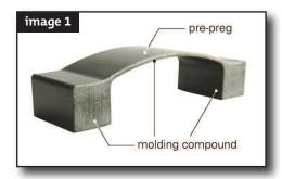
Despite this difference in the thickness of the bridge section, the redesigned part utilizing pre-preg showed a significant increase in the flexural performance, max load at failure and deflection at failure (Chart 1). In the redesigned pre-preg part, total failure (complete fiber break) was not observed but a delamination of the molding compound from pre-preg did occur (Image 2).
