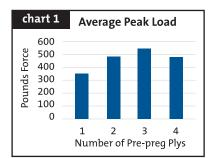
The part weighs approximately 0.20 pounds resulting in a load to weight ratio of more than 2,500.
