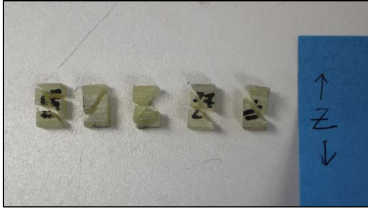
Figure 5: -150 C specimens post-test
