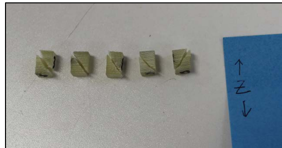
Figure 4: -100 C specimens post-test
