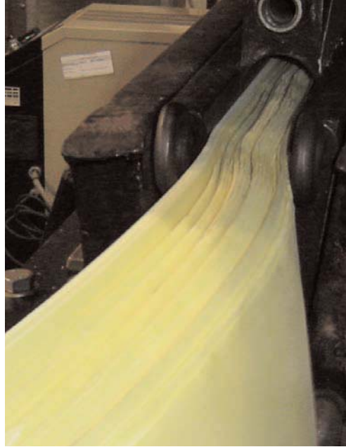
The process of creating thermoset composite rods, such as those that are used in the manufacture of the missile stabilizer, can be described in four basic steps. The first step is to load the prepreg material into the mold.
