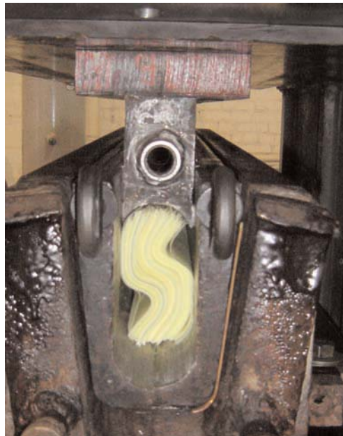
The above picture shows the thermoset composite material beginning to compress, which is the third step in the process.
