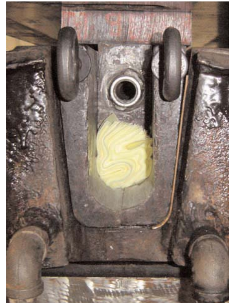
In the fourth step, the material begins to melt and flow into the final compression molded shape. The final product is a rod that will be ground and finished as required, then machined to the component's specifications.
