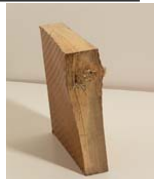
Side-view of fiberglass-phenolic laminate fired upon from close range with .50-caliber bullet.
